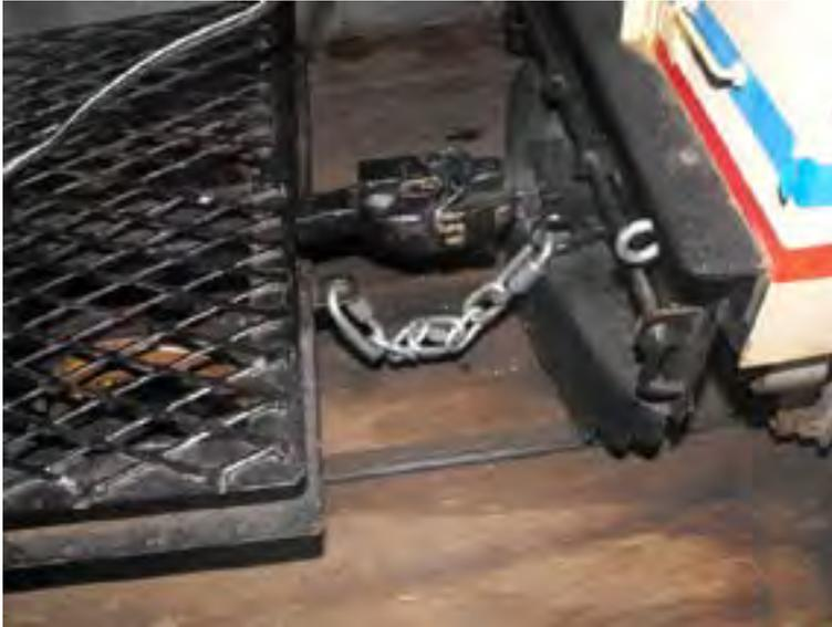
**This example shows a WELDED EYEBOLT on the locomotive on the right, and a TAB welded to the car on the left.**
