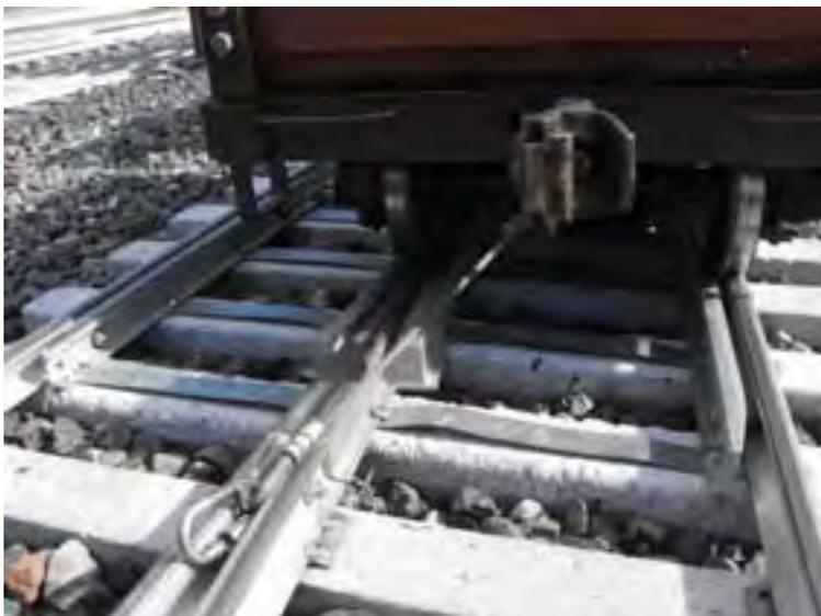
**This example shows what can happen when the free end of an unused safety cable or chain is not properly secured.**
