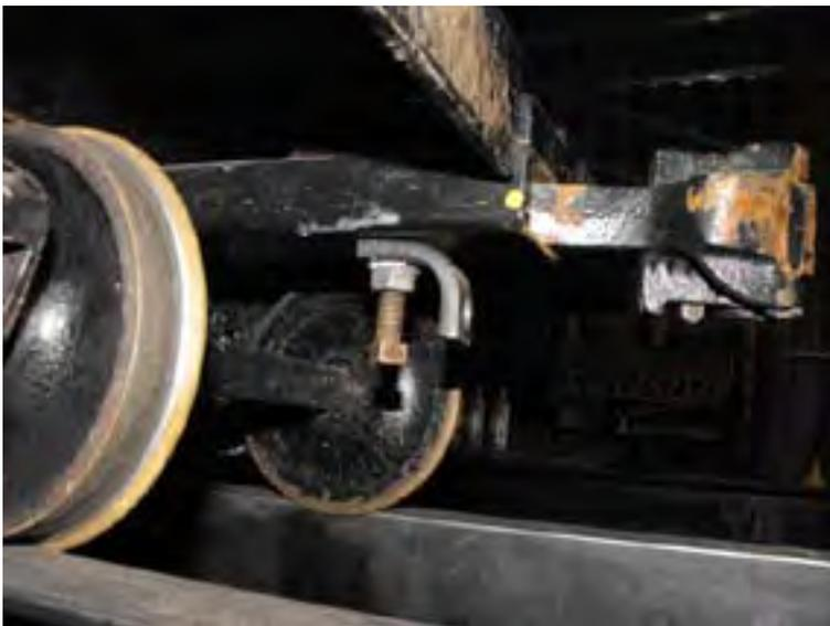
**This example shows a CONNECTION BRACKET which is BOLTED to the car.**
