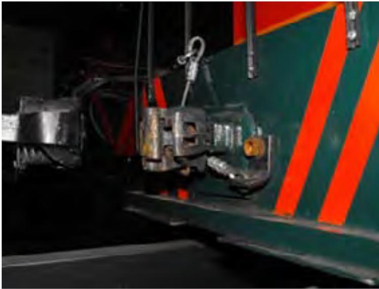
**This example shows a CONNECTION BRACKET which is BOLTED to a locomotive.**
