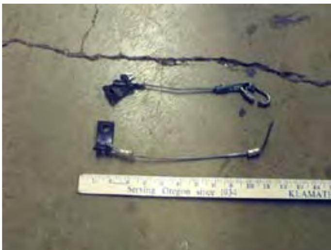
The top example shows a failure of the QUICKLINK. Most likely this was caused by the QUICKLINK not being screwed closed securely.
