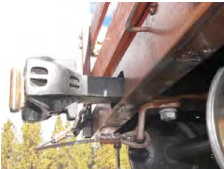
**This example Shows a CONNECTION BRACKET which is both BOLTED and WELDED to the car.**
