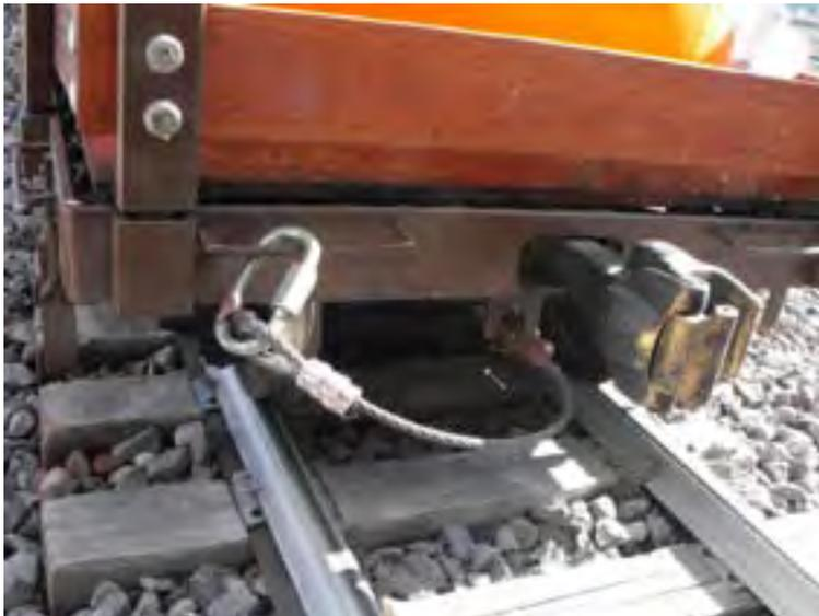
**This example shows a safety cable on the last car of a consist that is not in use, and it has the quicklink on the free end secured to the car.**
