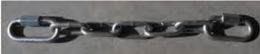
This example shows 3/16" WELDED LINK CHAIN, with 1/4" QUICKLINKS. Because the QUICKLINK is the weakest point, using the larger size makes this a good combination for heavy loads. It is **recommended** that the CHAIN be **no less than 3/16" WELDED LINK CHAIN**.
