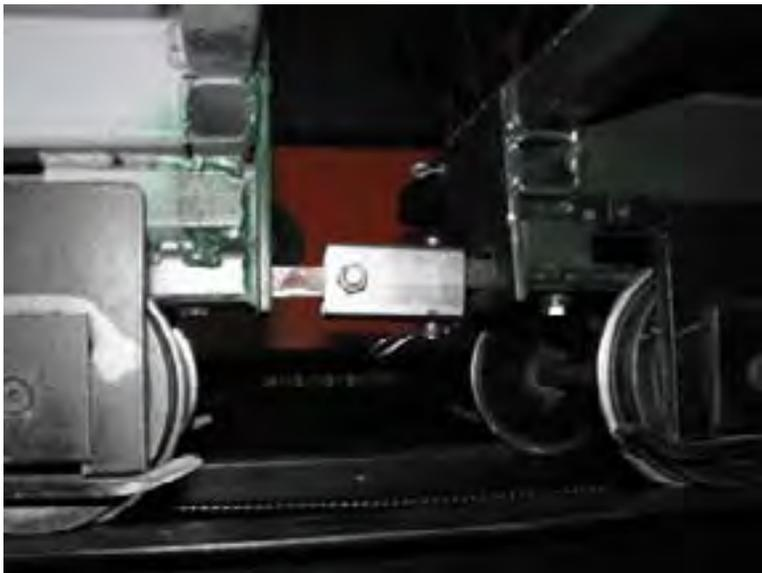
This is an example of one type of DRAWBAR. This particular setup features a DRAWBAR connection that pivots both up, down and sideways.
